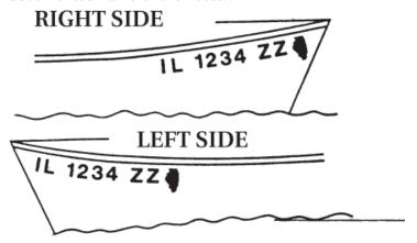
Hull Identification Number (HIN) Boats manufactured after 1972 will have a hull identification number consisting of 12 characters normally found on the outboard side of the transom, or if there is no transom, to the outermost starboard
